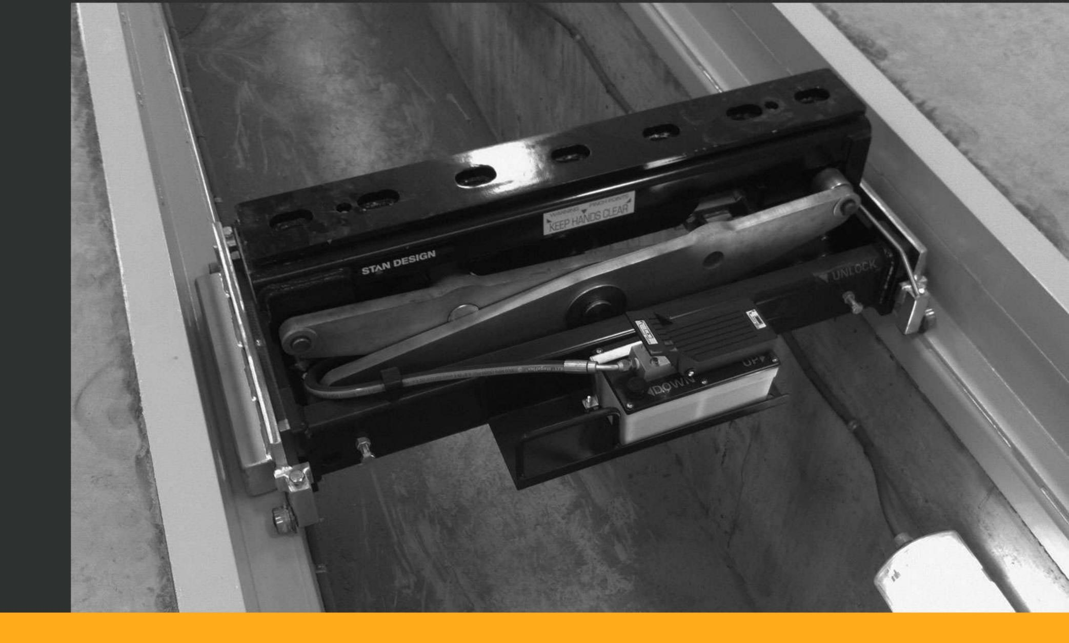
Turn your under-utilized inspection pit or lube pit into a full service bay with a PJ20DH Pit Jack
